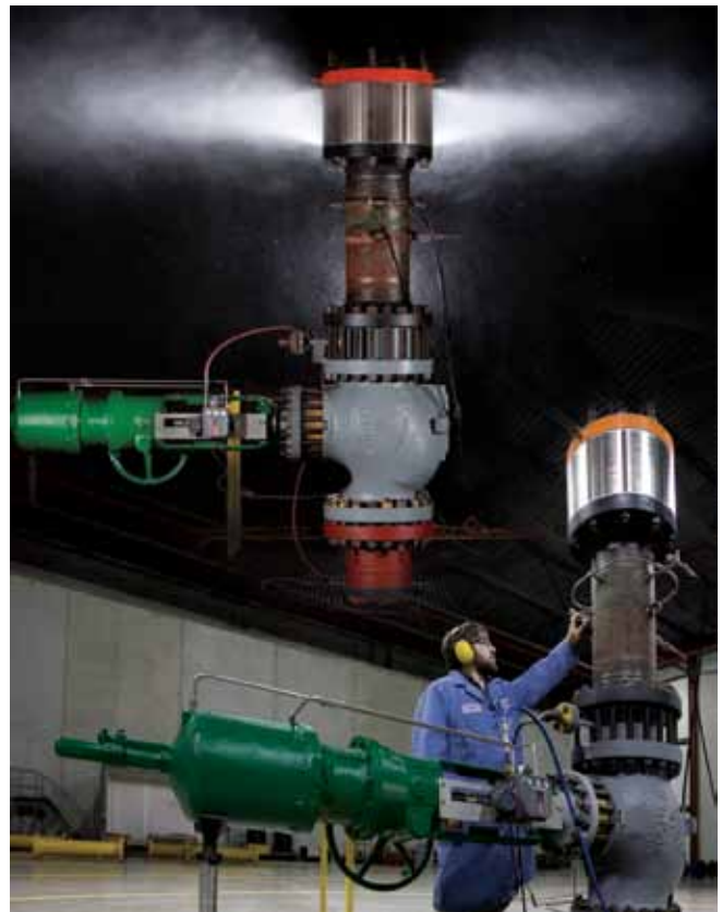
Noise testing of an NPS 12 vent diffuser.
