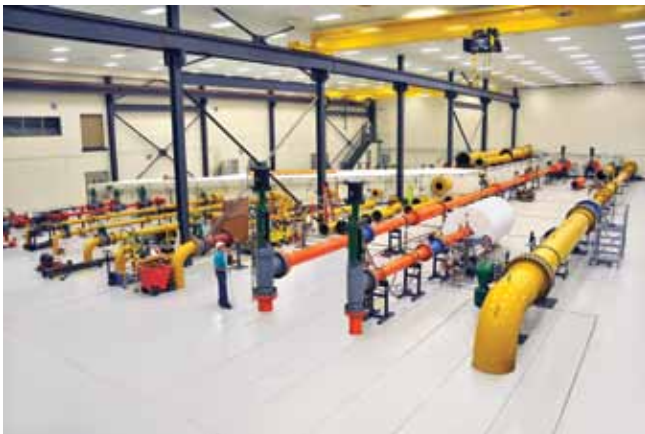
Fisher control valve designs undergo thorough and extensive flow testing in the 2,323 m 2 (25,000 ft 2 ) flow lab in the Emerson Innovation Center—the largest, most comprehensive control valve development center in the world.
