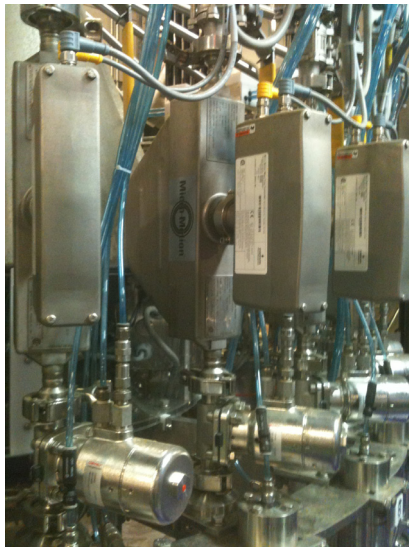
PSA 24-head filling machine with Micro Motion Coriolis meters with Filling Mass Transmitters
