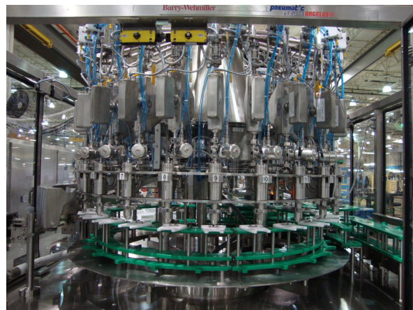
Mass-based filling machine with Micro Motion® Coriolis meters and Filling Mass Transmitters
