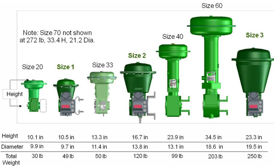
Figure 1: 1052 and 2052 Actuator Size Comparison
