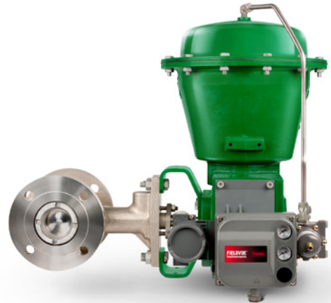
This Fisher CV500 rotary control valve features a contoured, segmented V-notch ball for throttling or on/off applications. The assembly also includes a Fisher 2052 size 2 actuator and a Fisher FIELDVUE DVC6200 digital valve controller.
