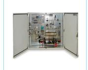
Precise high pressure bottle filling up to 12,000 psig / 1000 bar pressure for helium, argon and air. Meets cleanliness requirement to guarantee a bottle shelf life of 20 years.
