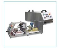
Automated design for leak testing hoses and hose assemblies with an accuracy and repeatability not possible using the manual test this unit replaced.
