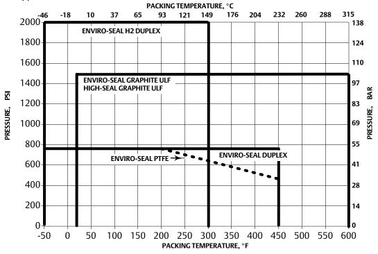
Figure 5. Applications Guidelines Chart for Nonenvironmental Service
