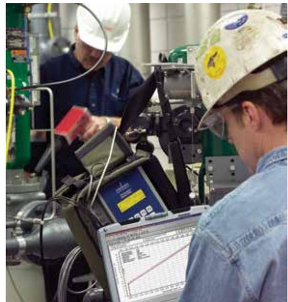
The portable FlowScanner 6000 is used to evaluate current operating conditions without having to disassemble or remove your control valves from the process. The FlowScanner system is flexible enough to run a variety of tests, including:
