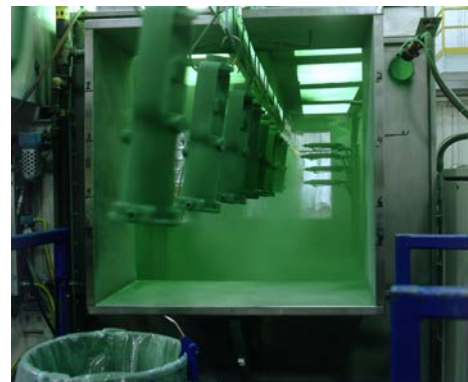
Figure 1. Powder Coating is Nearly 100% Free of VOCs
