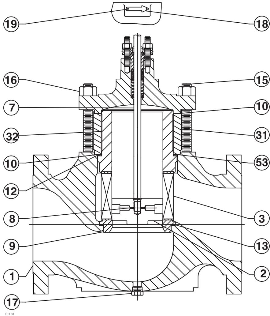
Keys 2\*, 7\*, and 8\* Valve Plug and Stem Assembly for Plain Bonnet
