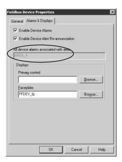
THE CONTROLLER IS ASSIGNED TO AREA A. A DEVICE THAT IS NOT YET ASSOCIATED WITH A CONTROL MODULE WILL DEFAULT TO THE SAME AREA AS THE CONTROLLER.
