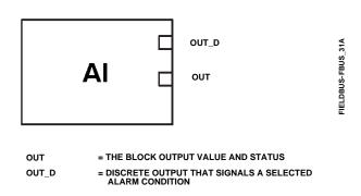
Figure 4-24. Analog Input (AI) Function Block
