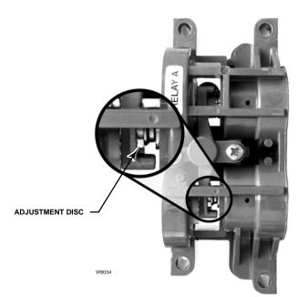
FOR SINGLE-ACTING DIRECT RELAYS: ROTATE ADJUSTMENT DISC IN THIS DIRECTION UNTIL IT CONTACTS THE
