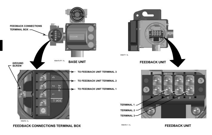
Figure 2-22. Terminal Details for Connecting Base Unit and Feedback Units of Remote-Mounted Digital Valve Controllers
