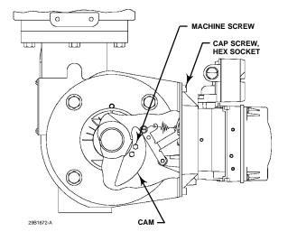
TYPICAL MOUNTING WITH SHORT FEEDBACK ARM (FISHER 1052 SIZE 33 ACTUATOR SHOWN)
