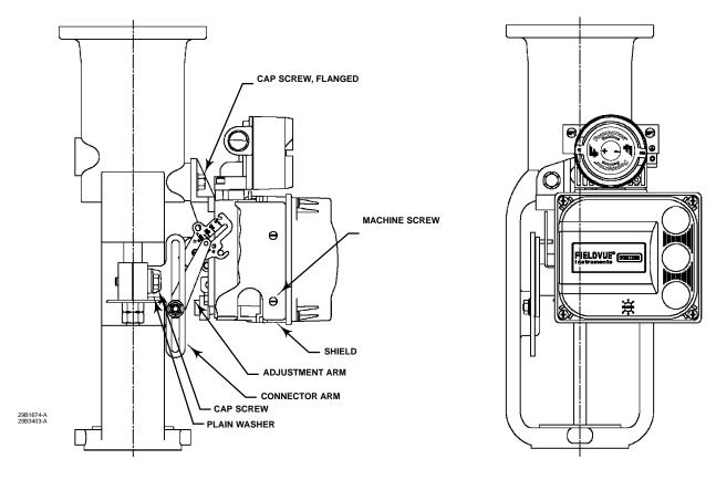
Figure 2-1. FIELDVUE DVC6010f Digital Valve Controller Mounted on Sliding-Stem Actuators with up to 2 Inches Travel
