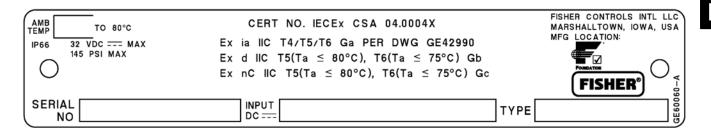
Figure B-20. Typical IECEx Nameplate for FIELDVUE DVC6010f, DVC6020f, DVC6030f, and DVC6005f
