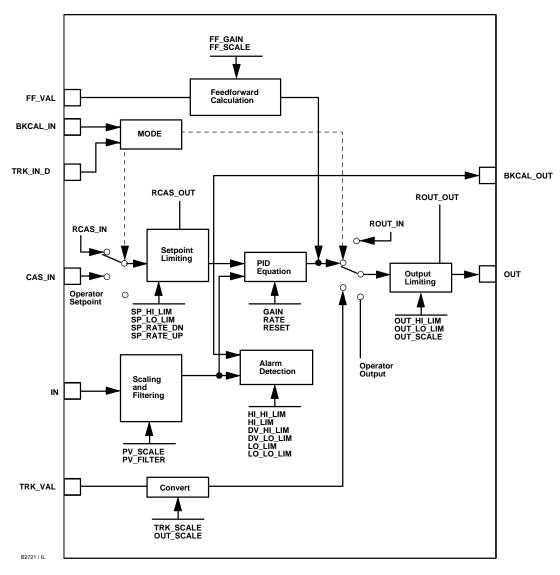
Figure 4-12. PID Function Block Schematic
