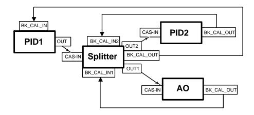
Figure 4-23. Output Splitter Configuration
