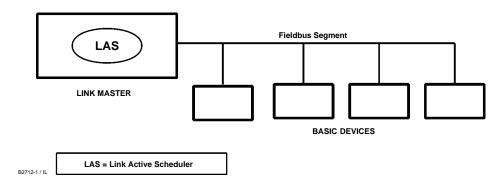
Figure D-3. Simple Single-Link Fieldbus Network
