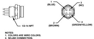
Figure 2-21. Quick Connect Connector
