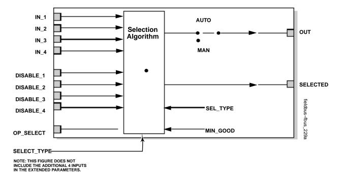
Figure 4-14. Input Selector Function Block Schematic
