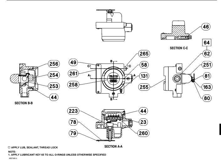
Figure 8-9. FIELDVUE DVC6035 Digital Valve Controller Assembly
