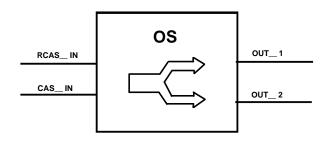
Figure 4-17. Output Splitter (OS) Function Block
