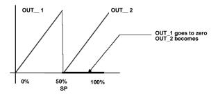
Figure 4-22. OUT with LOCKVAL False
