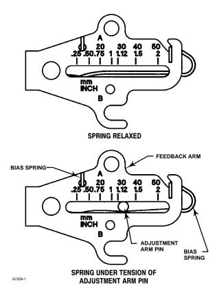
Figure 2-3. Locating Adjustment Arm Pin in Feedback Arm
