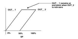
Figure 4-21. OUT with LOCKVAL True
