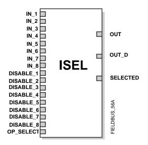
IN (1-8) = Input used in the selection algorithm.
