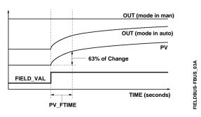
Figure 4-25. Analog Input Function Block Timing Diagram
