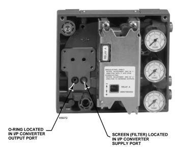
Figure 7-3. I/P Filter Location
