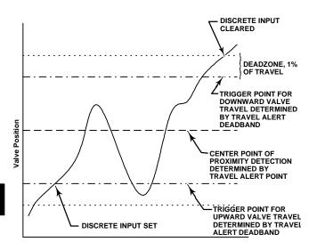
Figure 4-32. Discrete Input Proximity Detection Function
