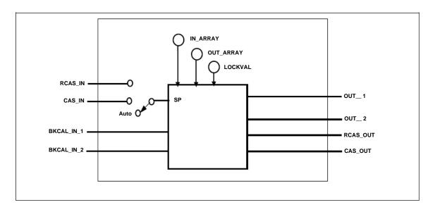
Figure 4-18. Output Splitter Function Block Schematic
