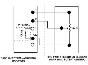
Figure 2-23. Terminal Details for Connecting a FIELDVUE DVC6005f Base Unit and a 10 kOhm External Potentiometer
