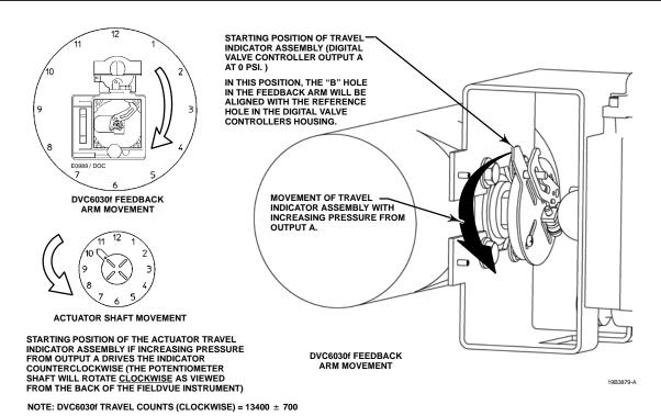
Figure 2-9. Explanation of FIELDVUE DVC6030f Travel Indicator Starting Position and Movement, if <u>Clockwise</u> Orientation is Selected for "Travel Sensor Motion" in ValveLink Software or the Field Communicator
