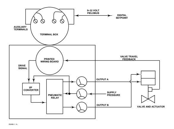
Figure A-1. FIELDVUE DVC6000f Digital Valve Controller Block Diagram
