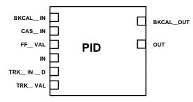
BKCAL\_IN = THE ANALOG INPUT VALUE AND STATUS FROM ANOTHER BLOCK'S BKCAL\_OUT OUTPUT THAT IS USED FOR BACKWARD OUTPUT TRACKING FOR BUMPLESS TRANSFER AND TO PASS I IMIT STATUS.
