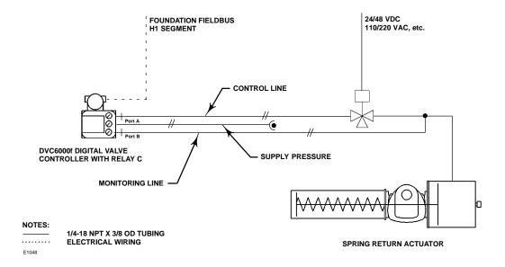
Figure 2-19. Pneumatic Hookup for Solenoid Testing
