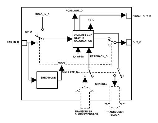
Figure 4-29. Discrete Output Function Block Schematic
