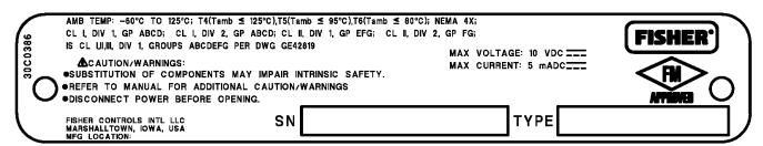
Figure B-9. Typical FM Nameplate for FIELDVUE DVC6015, DVC6025, and DVC6035
