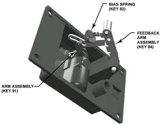
NOTE: INSTALL BIAS SPRING WITH SMALLER DIAMETER HOOK CONNECTED TO ARM ASSEMBLY (KEY 91) AND WITH BOTH HOOK OPENINGS TOWARD CENTER OF BRACKET.
