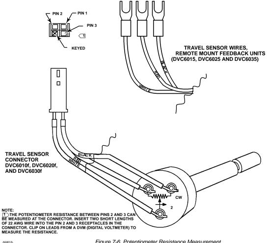
Figure 7-6. Potentiometer Resistance Measurement
