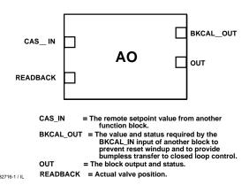
Figure 4-8. Analog Output (AO) Function Block
