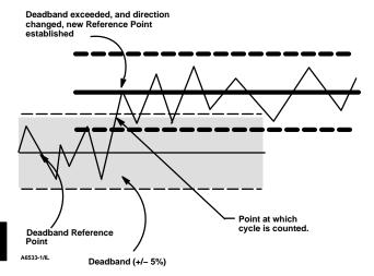
Figure 4-4. Cycle Counter Deadband (set at 10%)
