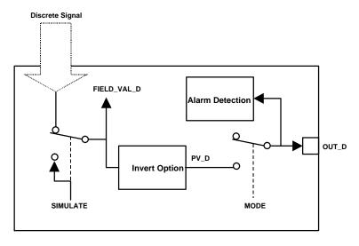
Figure 4-31. Discrete Input Function Block Schematic
