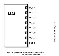
Figure 4-27. Multiple Analog Input (MAI) Function Block
