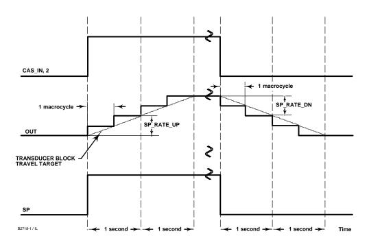
Figure 4-10. Analog Output Function Block Timing Diagram
