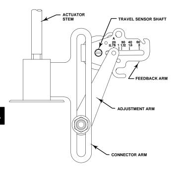
Figure 4-6. Feedback Connection for Typical Sliding-Stem Actuator (Up to 4 inch Travel)
