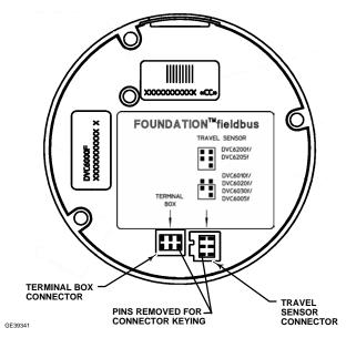
Figure 7-2. Back View of PWB Assembly Sub-Module
