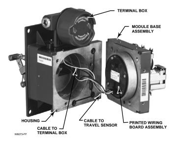
Figure 7-1. Printed Wiring Board Cable Connections
