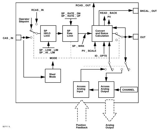
Figure 4-9. Analog Output Function Block Schematic
