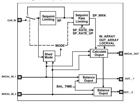
Figure 4-19. Output Splitter Function Block Schematic Diagram
