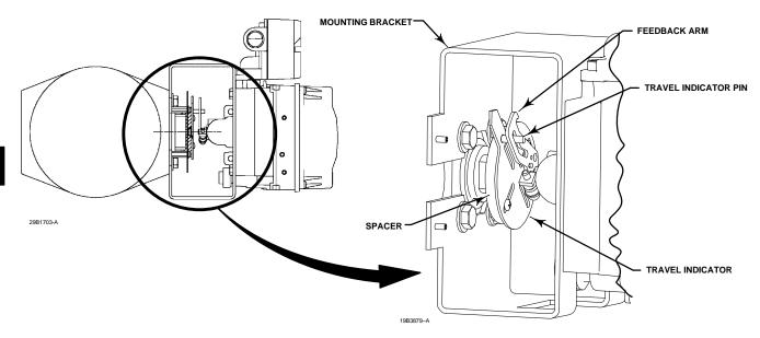
Figure 2-7. Mounting a FIELDVUE DVC6030f Digital Valve Controller on a Rotary Actuator (Fisher 1032 Size 425A Shown)
