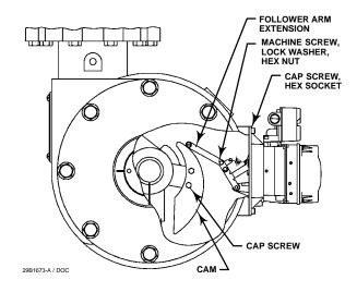
Figure 2-6. FIELDVUE DVC6020f Digital Valve Controller with Long Feedback Arm and Follower Arm Extension Mounted on a Rotary Actuator
