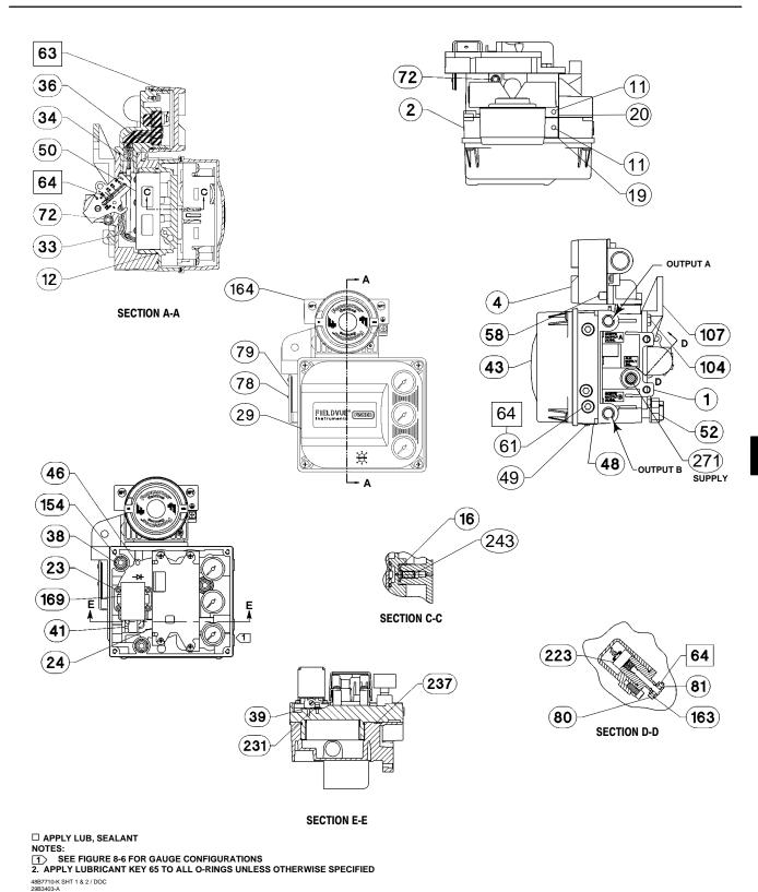
Figure 8-2. FIELDVUE DVC6010f Digital Valve Controller Assembly
