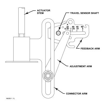
Figure 3-1. Feedback Connection for Typical Sliding-Stem Actuator (Up to 4 inch Travel)
