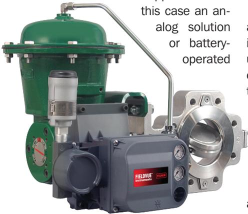
*Fisher® FIELDVUE™ DVC6200 with Smart Wireless THUM™ Adapter mounted on rotary valve assembly is an example of a digital valve controller that can provide specialized on-line diagnostics and communicate wirelessly.*
