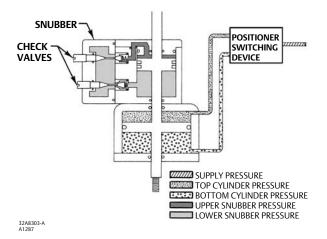
Figure 5. Operation of Actuator with Snubber
