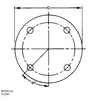
Figure 7. Dimensions for Actuators with Clevis Connection
