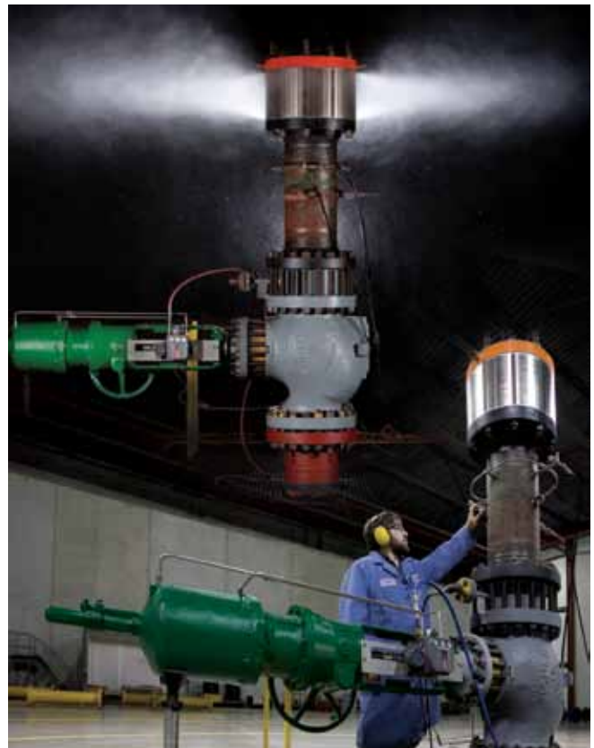
Noise testing of an NPS 12 vent diffuser.
