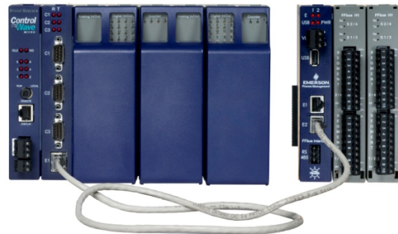
ControlWave Micro connected to the FOUNDATION Fieldbus Interface
