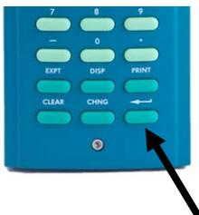
6. Select **TCP/IP Address 1**, provide a valid TCP/IP address, and press the enter key (located at the lower right corner of the keypad).
