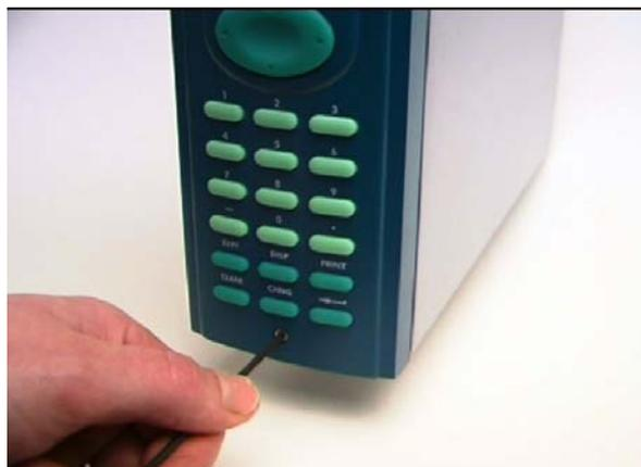
*Figure 1. Removing the Hex Cap Screw*
