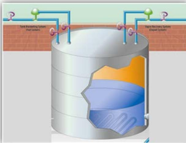
**Figure 4: Tank Blanketing and Recovery**
