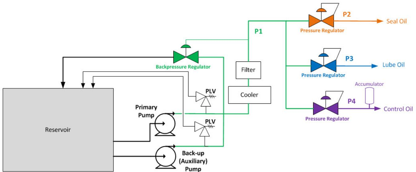
Figure 3: Lube Oil System
