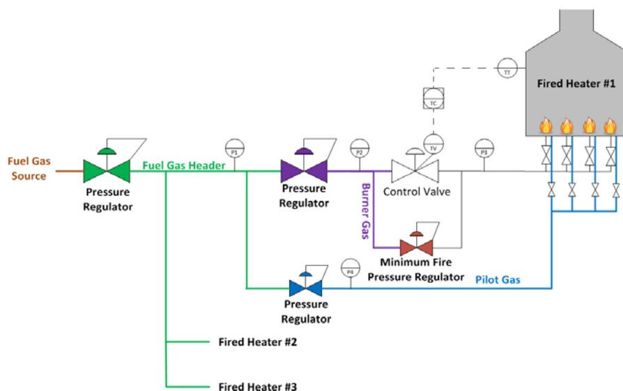
**Figure 2:** *Fired Heater Fuel Gas System*
