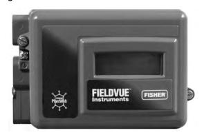
The high-performance linkage-less position feedback system eliminates physical contact between the valve stem and the digital valve controller or instrument. There are no wearing parts so cycle life is maximized. Additionally, the elimination of levers and linkages reduces the number of mounting parts and the mounting complexity. Digital valve controller or instrument replacement and maintenance is simplified because the feedback parts stay connected to the actuator.
