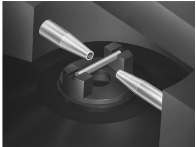
Figure 1. Detail of Deflector/Nozzle Pilot Stage
