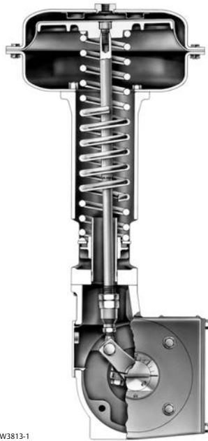
Figure 2. Sectional Views Typical of 1052 Actuator
