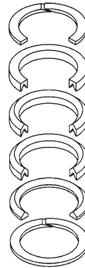
STACKING ORDER OF PTFE PACKING RINGS
