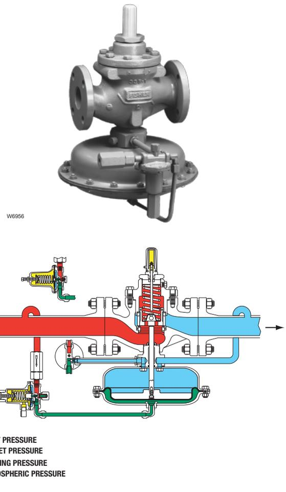
Figure 2. Type 1098-EGR Pilot-Operated Regulator and Operational Schematic
