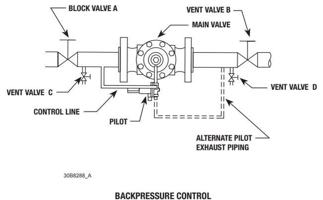
*Figure 5. Backpressure Regulator/Relief Valve Applications*
