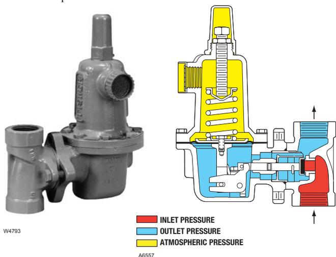
Figure 1. Type 627 Direct-Operated Regulator and Operational Schematic
