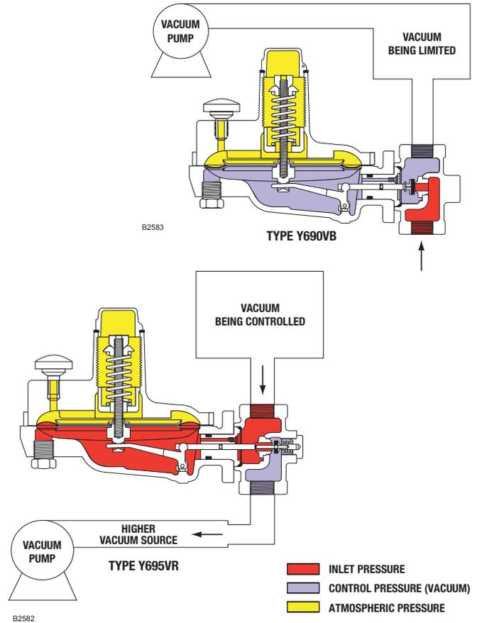
Figure 4. Type Y690VB Vacuum Breaker and Type V695VR Vacuum Regulator Operational Schematics
