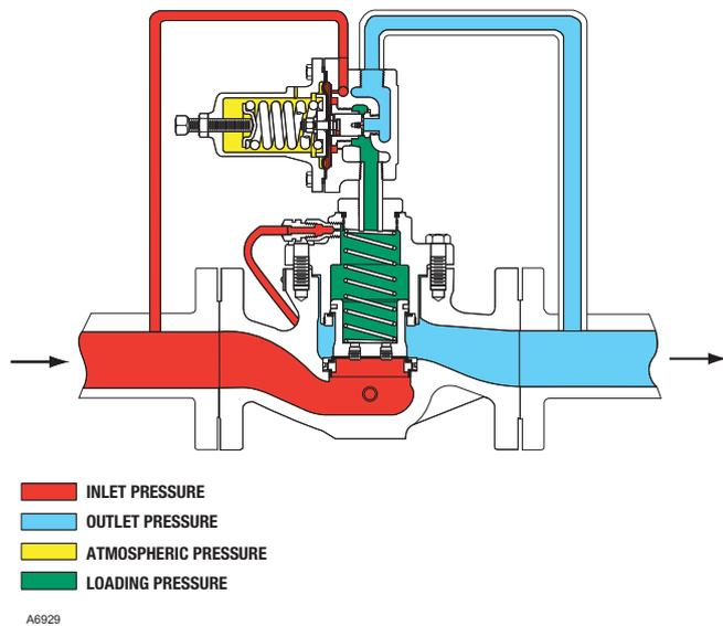
Figure 3. Type 63EG Backpressure Regulator/Relief Valve Operational Schematic
