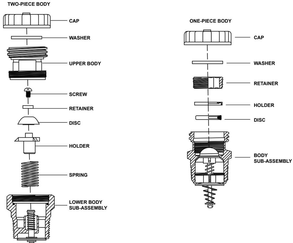
Figure 1. Exploded View of Typical Filler Valve Constructions
