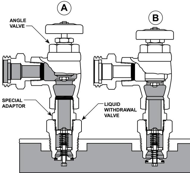
Figure 3. Operational Drawing of a Liquid Withdrawal
