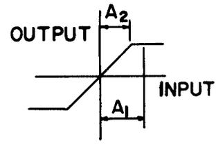
Figure 10. Describing Function for Saturation or Limiting
