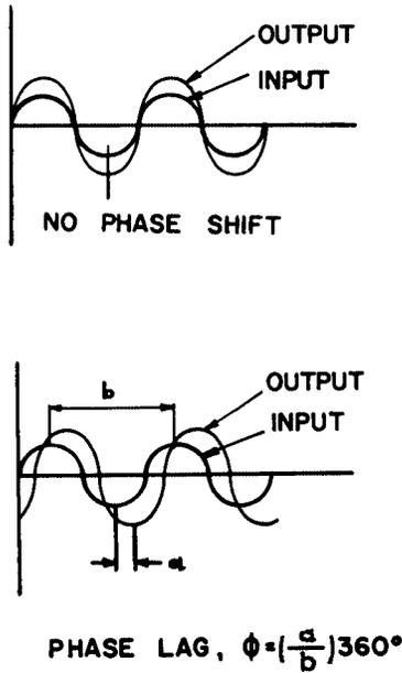
Figure 4. Measurement of Phase Shift
