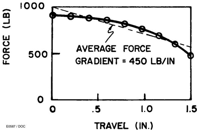
Figure 8. Typical Force Reaction on a Single Port Valve Due to Fluid Flow
