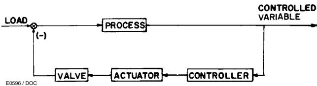
Figure 16. Block Diagram for a General Process Control
