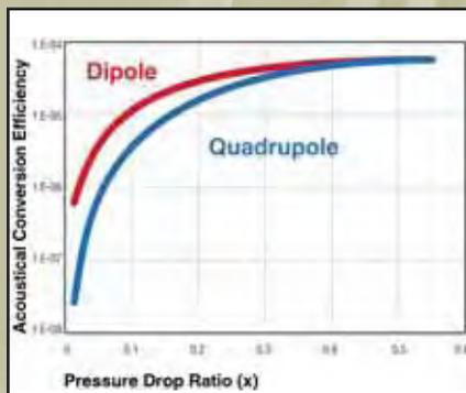
Therefore, it is important to keep flow within the quadrupole regime by keeping zones of high turbulent kinetic energy away from trim passage walls. (WhisperFlo trim also controls the location of turbulence relative to the valve body wall.) Controlling velocity alone is an impractical method to minimize noise.
