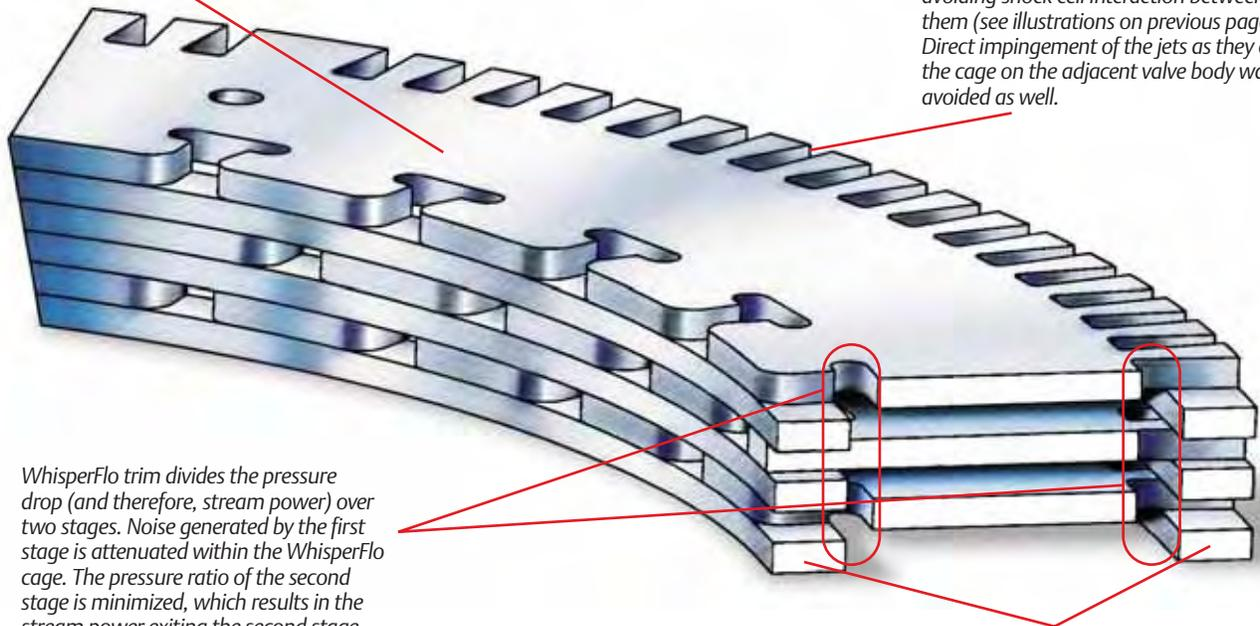
*WhisperFlo trim divides the pressure drop (and therefore, stream power) over two stages. Noise generated by the first stage is attenuated within the WhisperFlo cage. The pressure ratio of the second stage is minimized, which results in the stream power exiting the second stage being significantly less than that of a single-stage device.*
