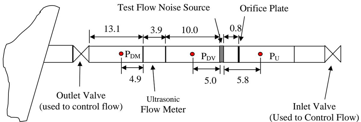
**Figure 2:** Schematic of the flow line. Dimensions are relative to a duct diameter
