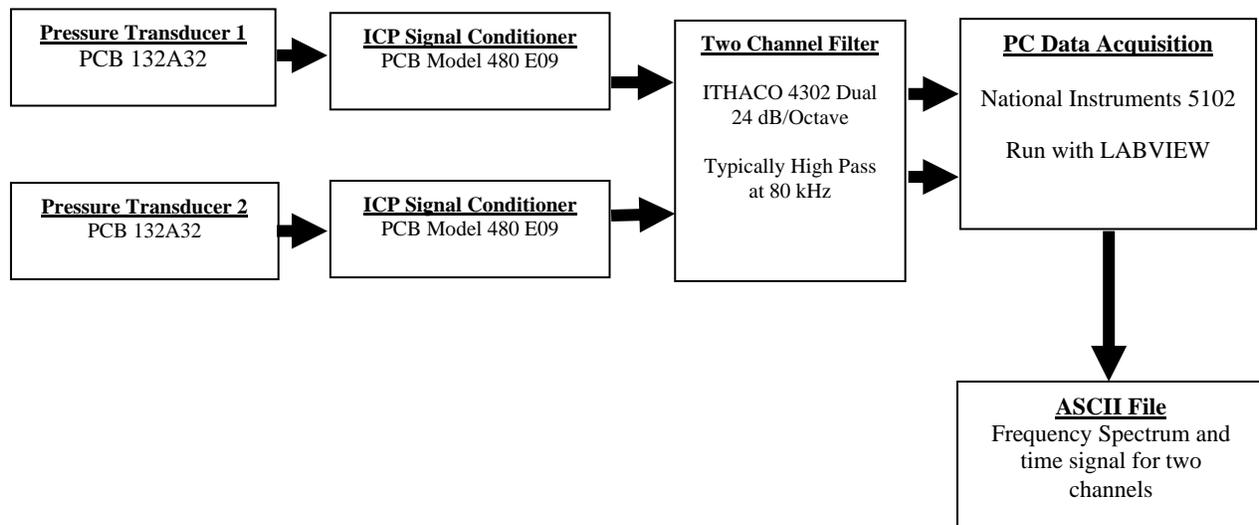
**Figure 1:** Diagram of the data acquisition system.
