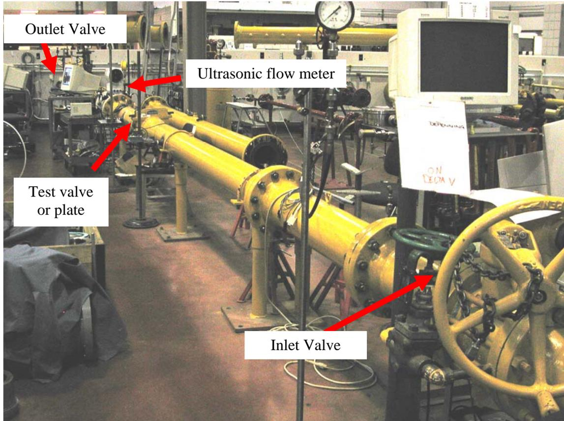
**Figure 3:** Picture of the flow line with key elements marked.
