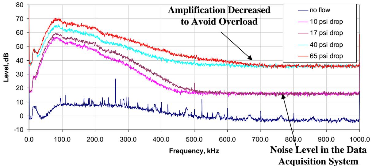
**Figure 4:** Example data down stream pressure,  $P_{DV}$ , of a plate with thirty five 1 inch holes.
