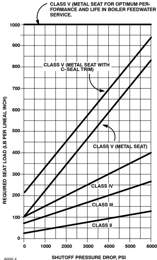
Figure 4. Minimum Required Seat Load for Metal Seated Valves.
