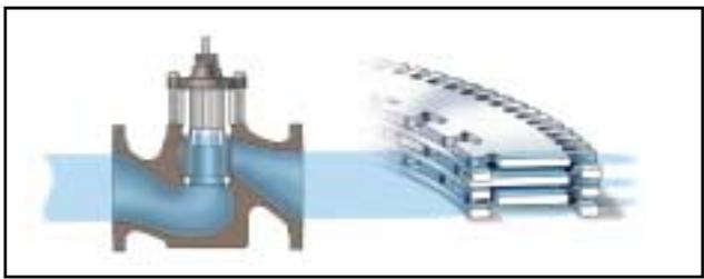
**Figure 3. Whisperflo: a recent innovation in noise abatement trim combines several principles to reduce noise, vibration and resultant pipe fatigue.**
