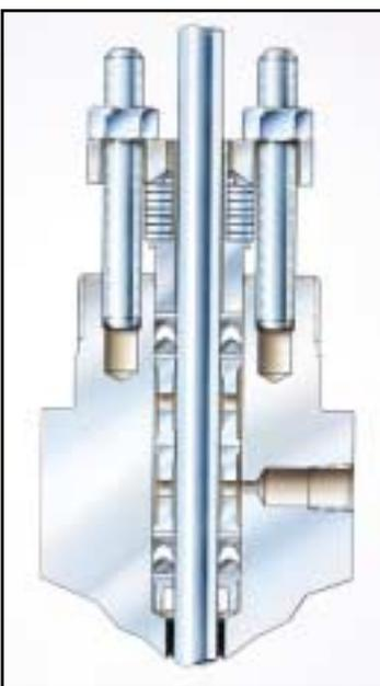
**Figure 2. Environmental protection in action. The Enviro-seal packing system reduces fugitive emissions and is an option on all Fisher valve bodies.**
