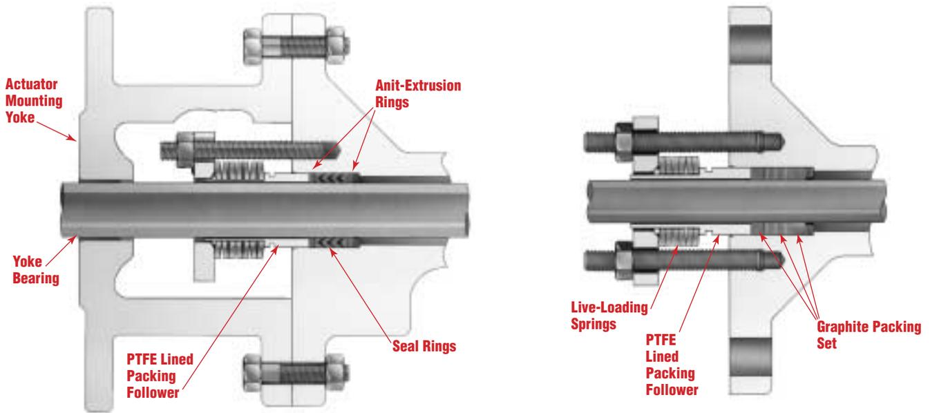
Figure 4: PTFE (left) and Graphite (right) packing systems for rotary valves.
