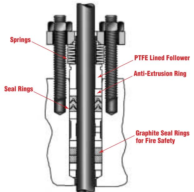
Figure 2: Duplex packing system utilizes both PTFE and graphite rings to provide emission control and fire safe operation.
