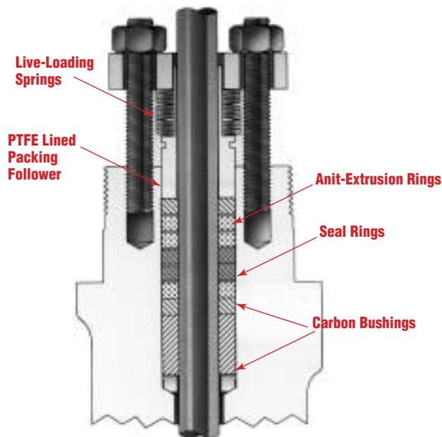
Figure 3: In contrast to PTFE-based system (Figure 2) the graphite emission-control packing system combines anti-extrusion rings, packing rings, and carbon guide bushings.
