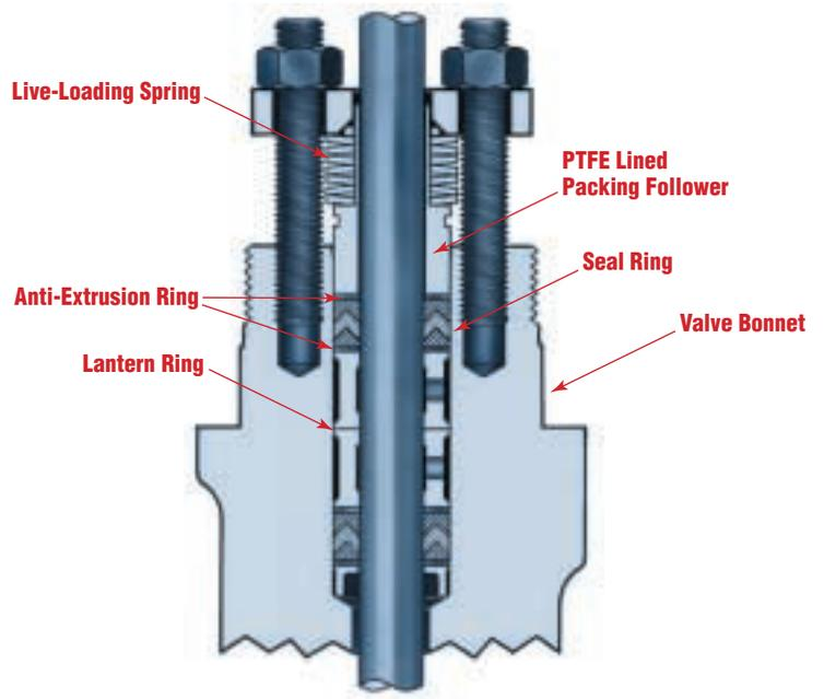
Figure 1: PTFE-based packing system features anti-extrusion rings above and below the packing ring set.
