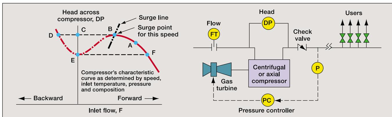
Fig. 1. Centrifugal-compressor performance curve showing key points in surge event and a simplified piping and instrument diagram of a compressor installation.
