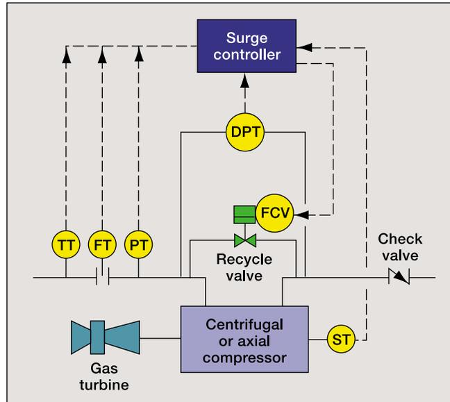
Fig. 2. Simplified piping and instrument (P&I) diagram of compressor installation with surge-control system.
