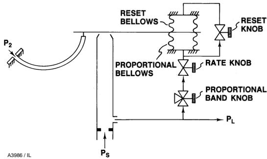
Figure 10. Proportional Plus Reset Plus Rate Controller
