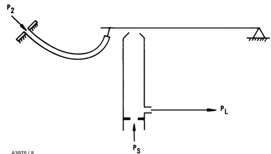
Figure 6. Nozzle-Flapper Amplifier with Bourdon Tube Sensor
