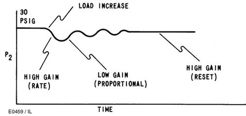
Figure 11. Control Performance with a Three Mode Controller
