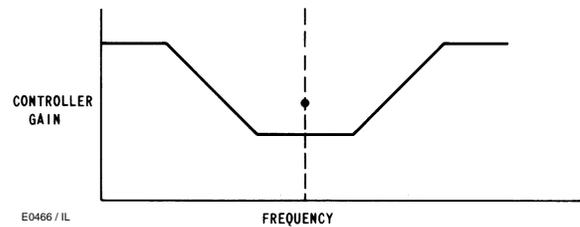
Figure 18. Properly Tuned Controller
