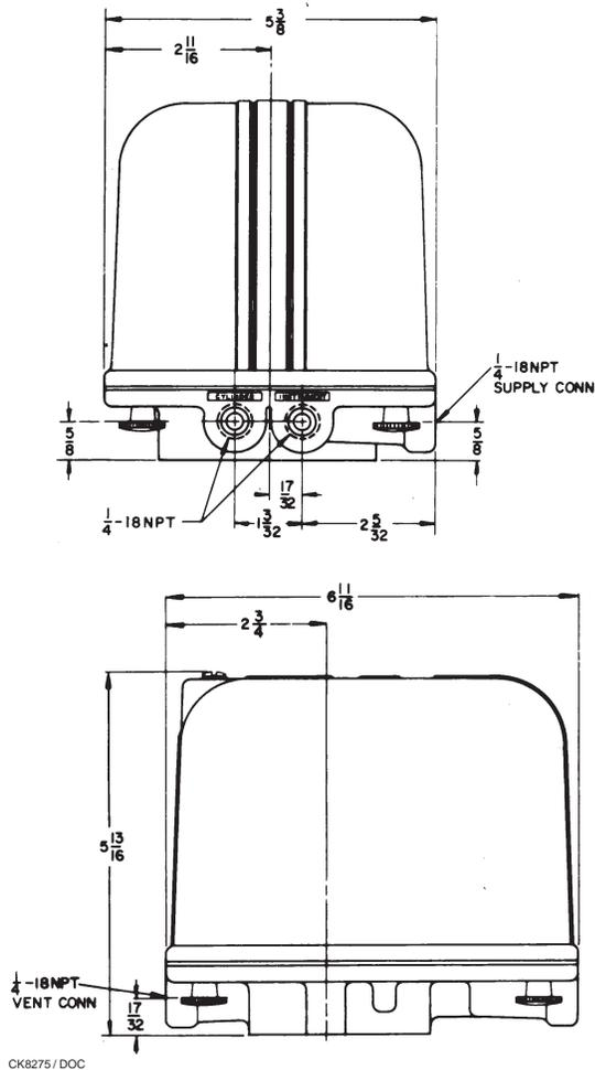
Figure 5. Positioner Connections
