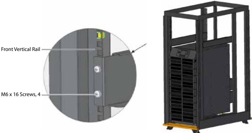
Figure 8: Securing the front of the rack-mount rails
