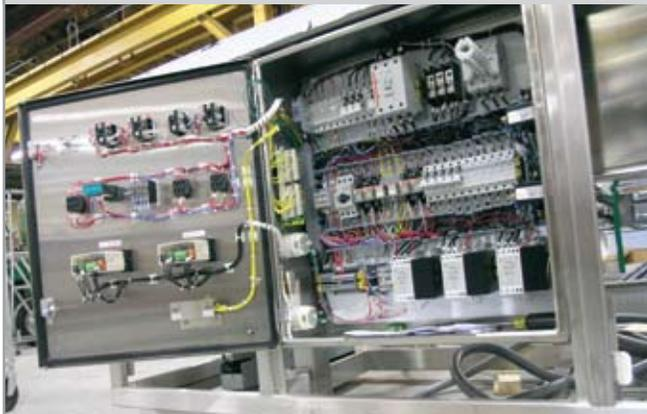
With the addition of an industrial PLC, all system functions can be controlled and monitored either locally or remotely. Basket bar coding can be added, eliminating manual operator input. Data acquisition can include bath operating temperatures, dwell times, liquid levels, pump flow rates, filter pressures, solution pH, conductivity, resistivity and ultrasonic power levels, etc., providing data that can be stored and retrieved as required.
