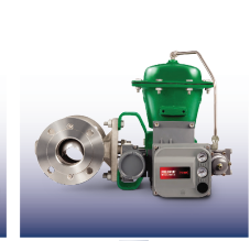
Vee-Ball™ valve Types : V150 & V300 DN25 to 200 and PN 10 to 40 NPS 1 to 8 and CL 150 to 300 WCC, 1.0619, CF3M SST, 1.4409 SST Types : V500 DN25 to 150 and PN 10 to 40 NPS 1 to 6" and CL 150 to 600 CF3M, WCC and WCC HT
