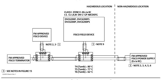
Figure 8. FM Loop Schematics—FIELDVUE DVC6200f and DVC6200p, FISCO Installations
