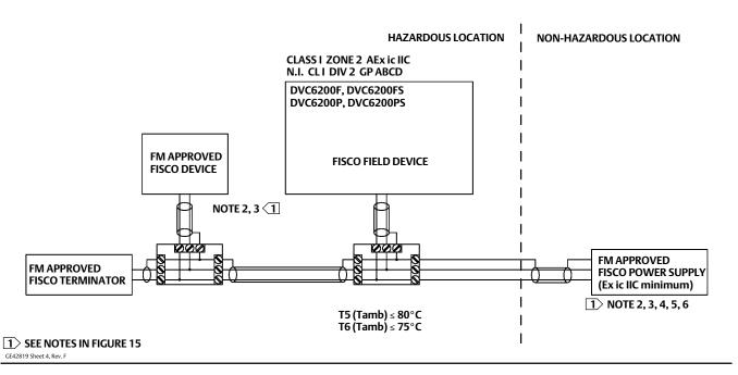
Figure 9. FM Loop Schematics—FIELDVUE DVC6205f, DVC6205p, and DVC6215, Entity Fieldbus Loop
