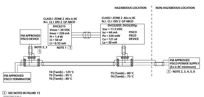
Figure 13. FM Loop Schematic—FIELDVUE DVC6200 HW1
