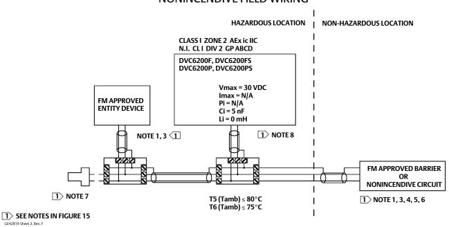
Figure 7. FM Loop Schematics—FIELDVUE DVC6200f and DVC6200p, FISCO Installations
