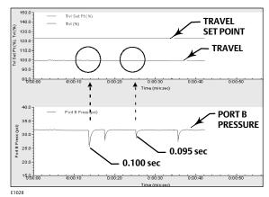
ValveLink Software Screen Image Showing Pressure Drop Across the Solenoid Valve
