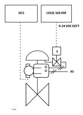
Figure 4. FIELDVUE DVC6200f Energize to Trip (ETT) and Solenoid Valve
