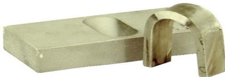
Figure 2: In foundry evaluation, a casting is filled with weld filler, then sliced to yield a bar for bend testing.
