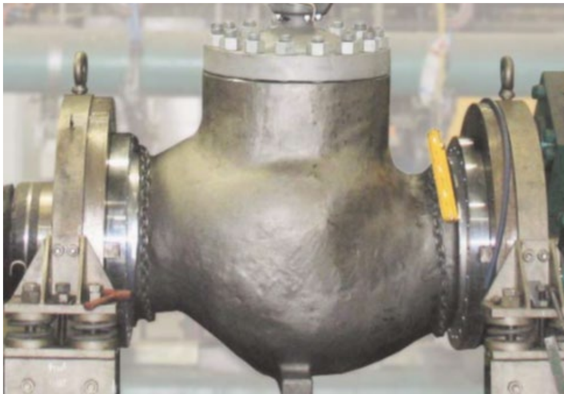
Figure 1: Pressure-retaining components of a valve are subjected to hydrostatic testing to evaluate the parts' integrity. Visible leakage or seepage through a casting means automatic rejection.
