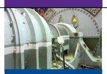
Wireless temperature, pressure, and DP have been employed to check for hot air leaks, forced draft fan leaks and filter plugging. Online monitoring has enabled engineers to improve turbine efficiency and reduced megawatt use as well as extend the life of turbine fans.
