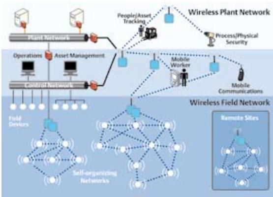
*Out in the field, the self-organizing ability of wireless mesh networks, such as used in WirelessHart, moves into action when an established signal path is blocked.*
