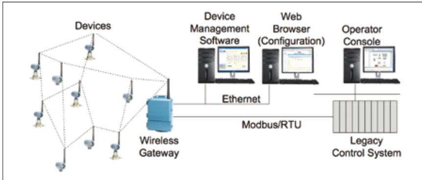
A wireless gateway enables legacy control systems to receive process variables from wireless transmitters.
