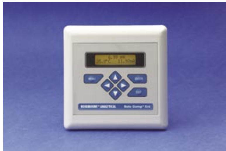
Figure 1: pH analyzer supports EDDL for remote management.
