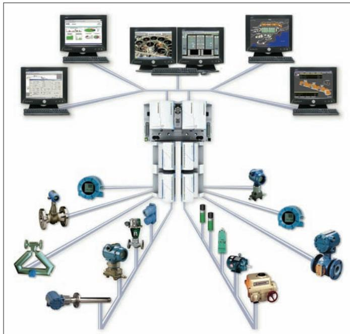
**A digital plant architecture incorporates high-speed communications networks, intelligent field devices, and bus I/O technologies to offer unprecedented insight into operations at a single plant or across multiple plants within a municipality's operations. Photo by Emerson Process Management**
