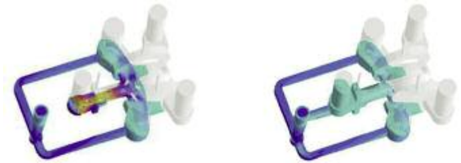
Figure 7. In the two-feeder casting method (left), a high level of turbulence was created as the metal flowed into the neck and foot. The three-feeder casting system resulted in tranquil and low-velocity fill.
