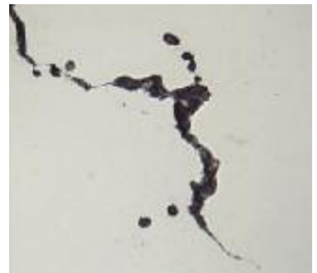
Figure 4. Photomicrograph showing the leak path and the continuation of the grain boundary. Original magnification 500x.
