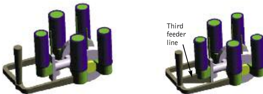
Figure 6. Casting rigging with two-feeder method at left and three-feeder method at right
