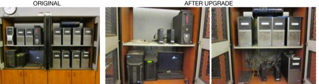
Virtualization enabled plant to remove significant hardware from behind the control-room workstations
