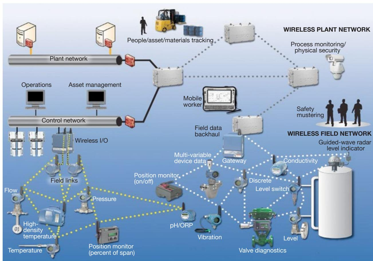
1. All of the typically measured parameters important to control and M&D can be monitored wirelessly with today’s technology
