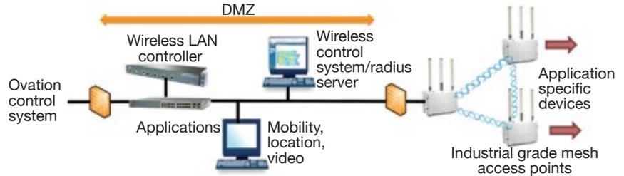
**2. The three “buckets” of a wireless system:** (1) Field devices/links communicating through a mesh wave field; (2) the infrastructure level, a wireless LAN controller, server, and terminal to collect and manage the data and RF requirements; and (3) the applications
