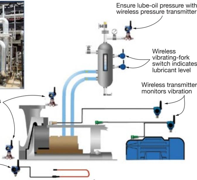
**4. Wireless M&D options** for a single pump include filter monitoring (pressure), leak detection, vibration monitoring, level sensing, and lube-oil pressure
