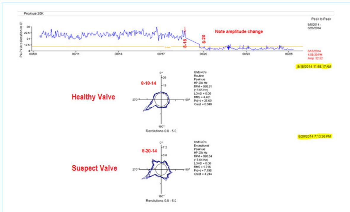
Let's first look at the trend value. Given the fact that we are dealing with a form of flow turbulence instead of impacting, what we notice is that the amplitude actually decreases when a valve is not properly sealing. This is due to the fact that the Delta Pressure is less across an improperly functioning valve, the usual "surge" of gas as the valve opens and closes is substantially reduced.
