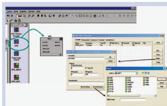
**FIG. 3** Modern APC applications are graphically configured with prebuilt function blocks and built-in tag browsers.
