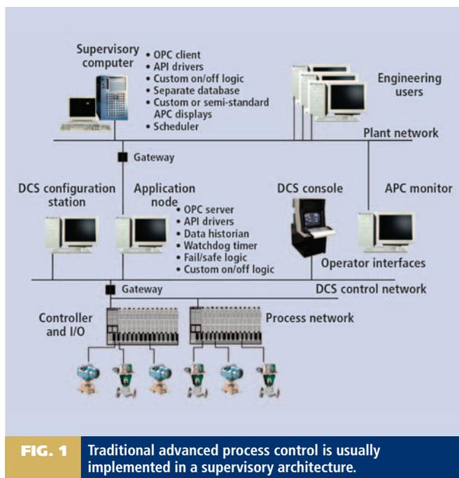
**FIG. 1** Traditional advanced process control is usually implemented in a supervisory architecture.
