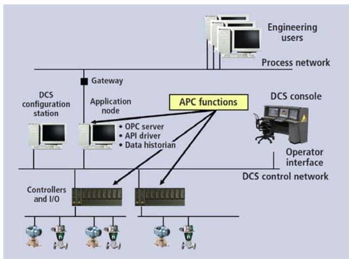
**FIG. 2** In an embedded advanced process control architecture, functions can be distributed and executed on multiple controllers or application stations running on the native control system bus.
