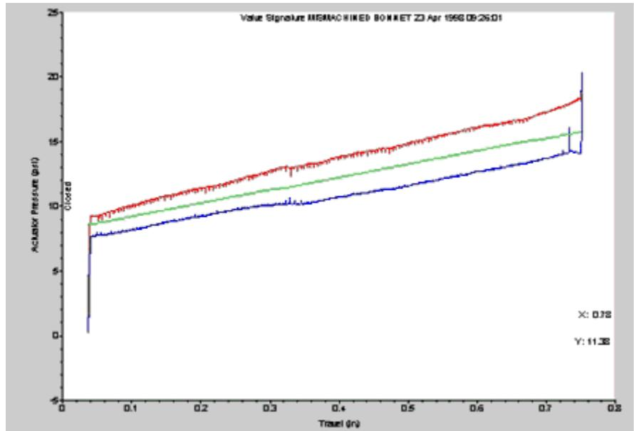
In the past, detecting stiction required taking the valve off-line to perform a “bump test.” With ValveLink technology, you can check for changes in signature while the valve is still in service, making it much easier to detect problems before they affect product quality.
