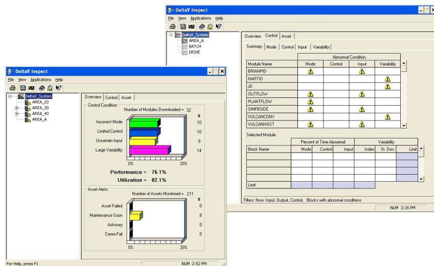
When the problem is a poorly tuned loop, easy but powerful **DeltaV Tune** software uses patented relay oscillation principles that minimize process disturbances and minimize tuning time. **OvationTune**, a system-wide tuning package, smoothes out variability by monitoring and adaptively tuning loops for optimal performance.
