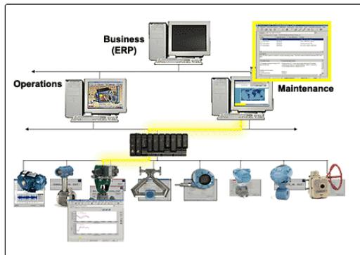
Diagnostics at the valve are continually monitoring the drive signal of the I/P and are able to detect when dirty air **starts** to clog the I/P. The valve is still operating correctly, so there is no need to notify the operator. This predictive situation is sent to the Maintenance department for a solution.
