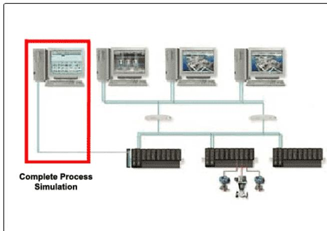
Simulation software should be non-intrusive and provide real-time process modeling. This allows you to test your control strategies without affecting your actual process.
