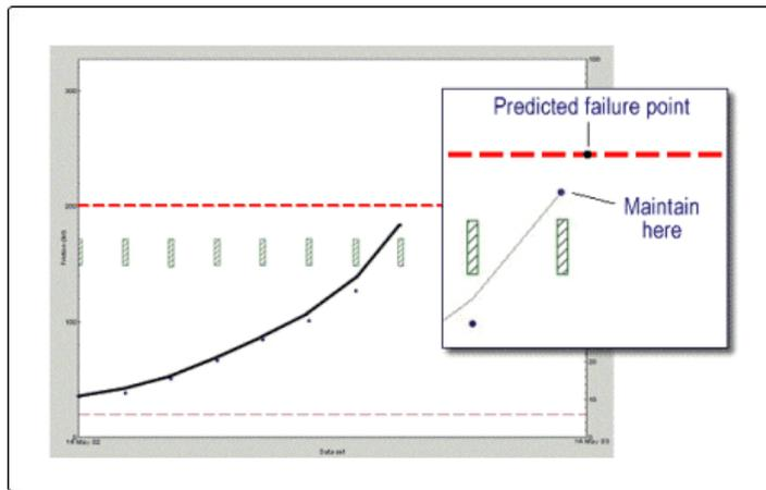
Digital predictive intelligence provides early warning of potential problems. This valve diagnostic, for example, indicates that friction will exceed the recommended limit in one month, enabling you to schedule replacement of the valve packing before deteriorating performance affects safety, health, or environmental protection.
