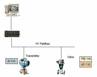
A simple device may have only a single input or output function block. More-complex devices may have several input and output blocks, as well as blocks for monitoring and control.
